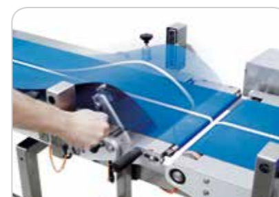
Easy feeding belt removing for cleaning
